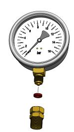
No loss connector is supplied only with gauges rated up to 25bar. When using no loss connector make sure to use supplied seal, otherwise the gauge will not work correctly.
