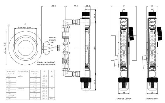
Typical Pipeline Configuration (Horizontal or Vertical)
